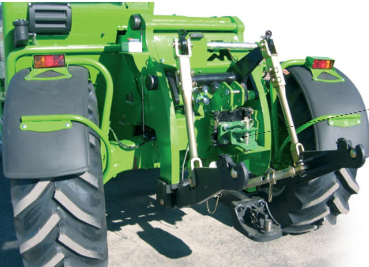
The rear towing hook may permit the towing of trailers and agricultural implements with a towing mass of up to 20 tonnes, where local transport regulations permit.
