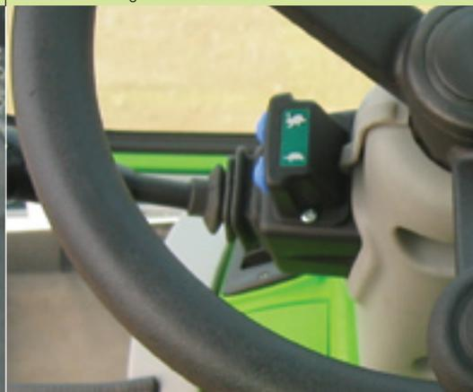
The electro-hydraulic 'Finger-Touch' reverser allows the operator to reverse driving direction without even taking his hands off the steering wheel.
