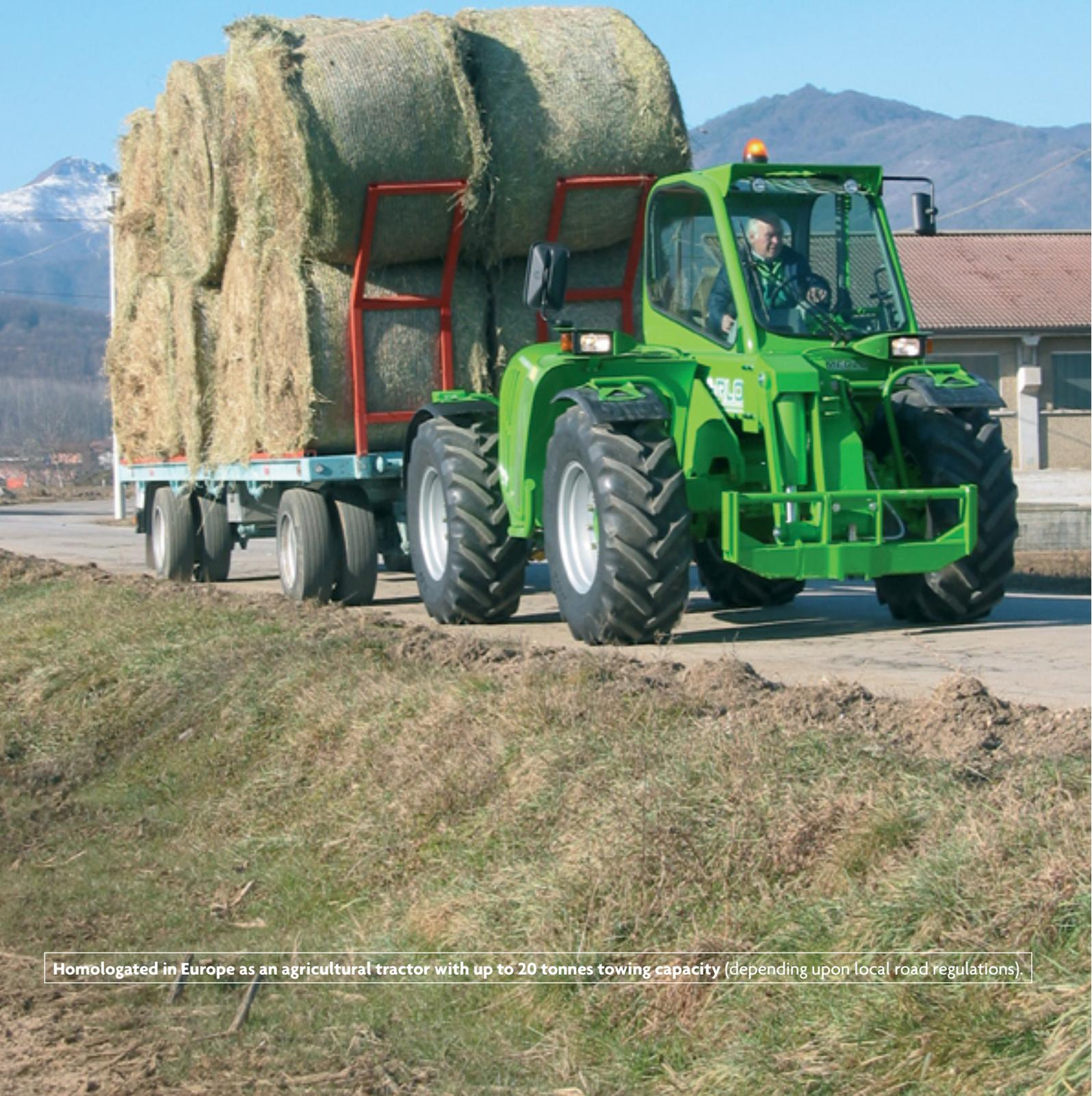
Homologated in Europe as an agricultural tractor with up to 20 tonnes towing capacity (depending upon local road regulations).
