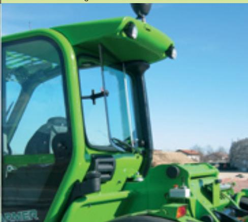
The wide glass surface area of the cab ensures truly panoramic visibility. The front and rear windows, and the upper door section, can be opened for 'natural' ventilation.
