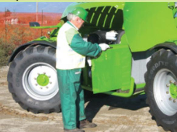
The engine can be swung away from the chassis for easy maintenance.
